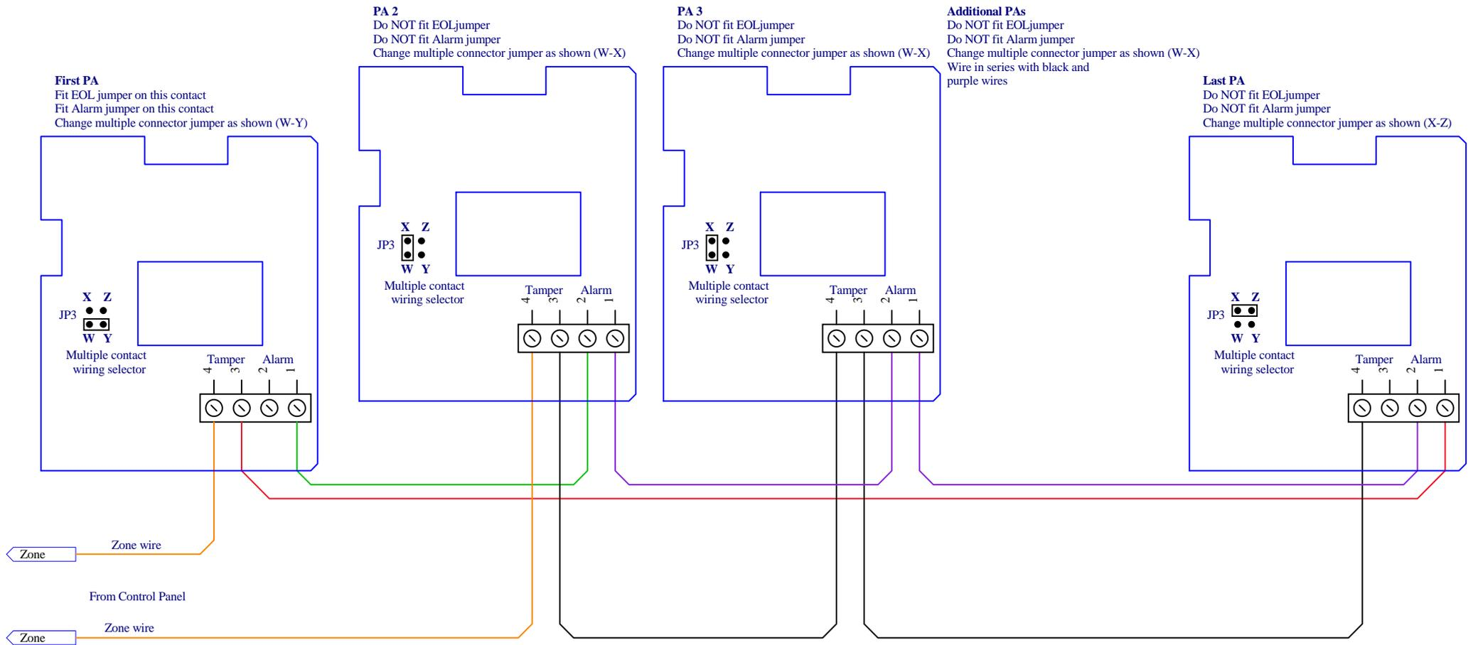
Wiring multiple PA2 Panic buttons in series, both protected by tamper circuits, for a grade 3 EOL loop
