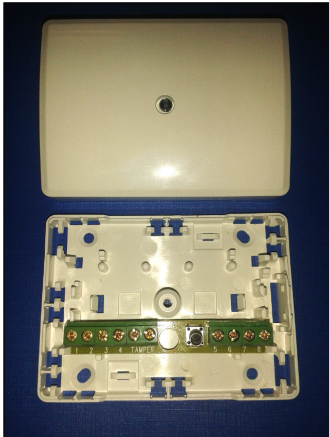
Fig. 1 – J10 Junction Box
