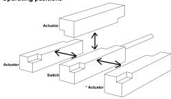
Sensor and the three possible operating faces for the magnetic actuator which should move parallel to the sensor
