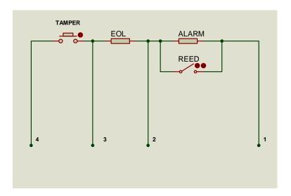
The ALARM PANEL monitors the contacts, usually one contact for each zone, and will be expecting three resistance values. It is connected to the contact at terminals 1 and 4. Terminals 2 and 3 are used where a different configuration is required eg no TAMPER or no EOL.
