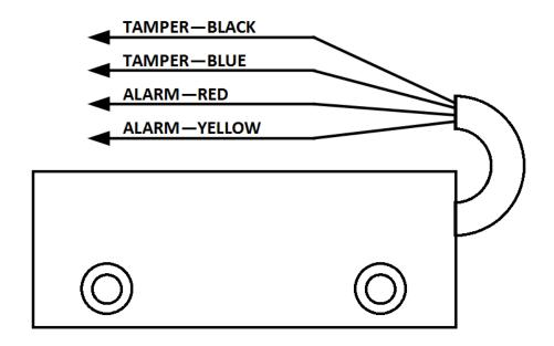
When wiring is to the desired specification, fit the contact to the mounting holes using the screws provided. Ensure that contact & magnet align as well as possible to ensure reliable operation.
