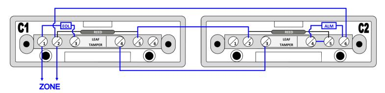
Link C1,T1 and C1,T2 to Zone Link C1,T1 and C1,T3 to EOL Resistor
