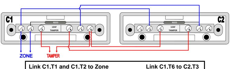
Link C1,T1 and C1,T2 to Zone Link C1,T3 and C1,T6 to Tamper Link C1,T4 to C2,T4 Link C1,T6 to C2,T3 Link C2,T2 to C1,T1 Link C2,T5 to C2,T5
